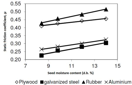
**Figure 10.** Relationship between static friction coefficient of variety Shirin and moisture content
