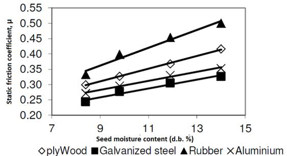
**Figure 11.** Relationship between static friction coefficient of variety 436 and moisture content
